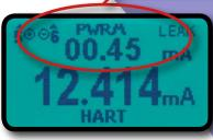
**Built-in troubleshooting tools** Detect hidden loop problems caused by ground faults & current leakages.
